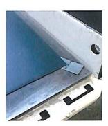
To Measure the planarity, it is necessary to insert into the empty space between the corner and the comparison plate, a steel thickness gauge presents in the end of production line, beyond kiln.
